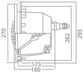
Diamond Pool Light Plastic Niches are concrete pool light niches molded of high-strength corrosion resistant PVC with a -lin. PVC hub.
